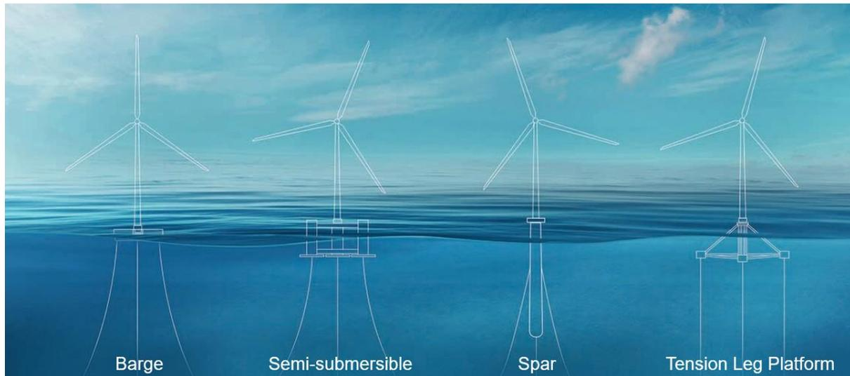
Figure 6: FOW Foundation Types [Image Credit : DNV GL]
