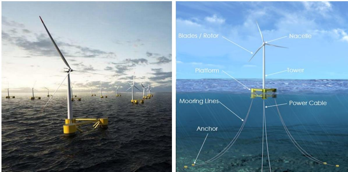
*Figure 1 - Floating Offshore Wind Platforms & Key Components*
