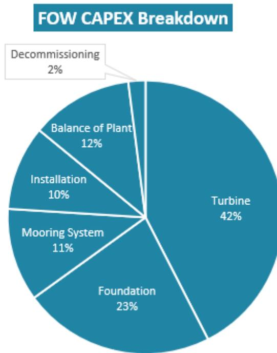
Figure 4 - Cost breakdown for typical fixed & floating offshore wind projects (source: Carbon Trust)
